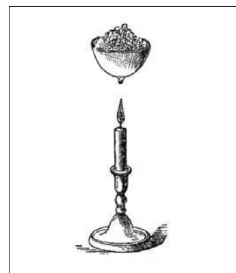
Figure 2 – Assembly designed to collect a drop of water produced by the candle’s combustion. (Faraday, 2002, p. 66)
